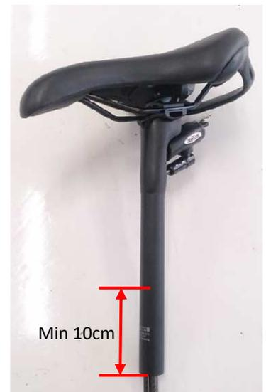
2.3.3 Adjust saddle to proper height and face forward, then closure seat clamp.
